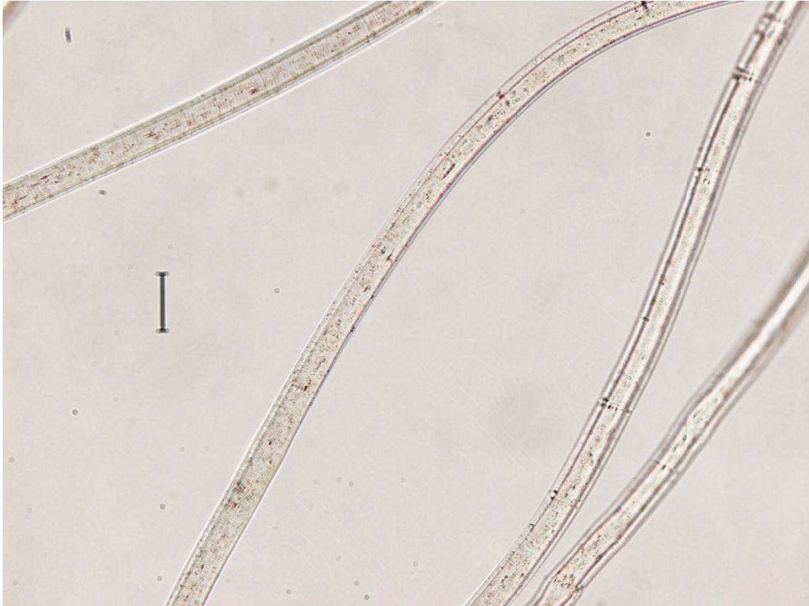
Ph. 2-29 Example of a core/sheath bicomponent fibre type.
