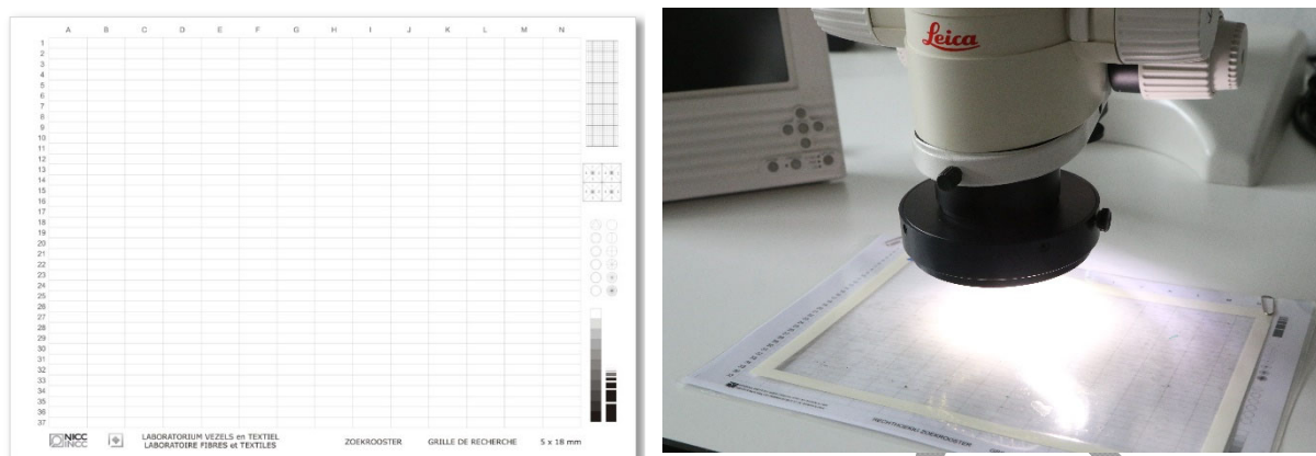
Fig. 1-6 Screening of tapings using a search grid.
